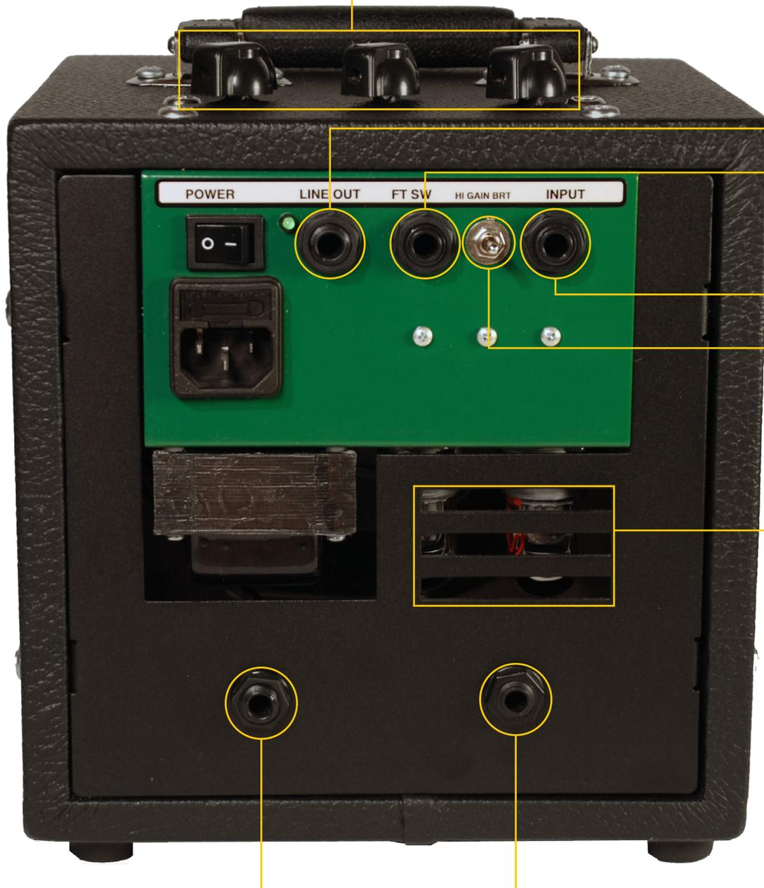
**Line Out** - The line out can be used either as a traditional line out for recording or its second purpose is an effects loop utilizing a TRS cable.
